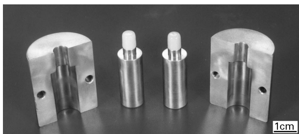
Figure 2 Split brass mould for making complete crown shapes with Vita Alpha dentine porcelain for In Ceram and for casting wax crown shapes for OPC TM and IPS Empress. Samples of In Ceram complete crown shape on the centre right and OPC TM on the centre left are also shown.
